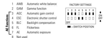
Figure 1. Switch Settings for Varifocal Lens
